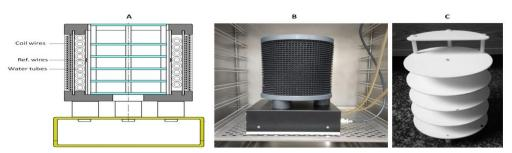
**Figure 2:** The intermediate frequency exposure system. A: scheme of the solenoid IF exposure system. B: the solenoid coil exposure system placed in the  $CO_2$  incubator. C: sample holder within the solenoid coil.
